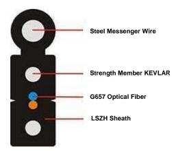
Suitable for self-supporting aerial and duct FTTX Drop Installations. Able to transmit all wave lengths.
